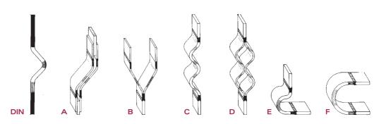
SHEETS OF DRILLINGS For connection between expension connectors and busbars (see DIN 46 206 resp 43 673)
